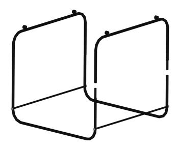
**B.** Slip the ends of the upper support fully into and over the uprights of the lower support section. Repeat with the second support. *Continued...*
