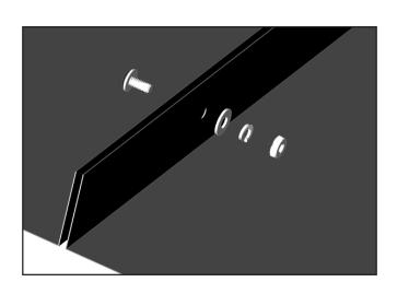
**B.** Fasten Segment A to first Segment B using: 1 #10 Bolt (silver) 1 #10 Flat Washer 1 #10 Lock Washer 1 #10 Hex Nut at each of the five holes. Hand tighten all bolts.
