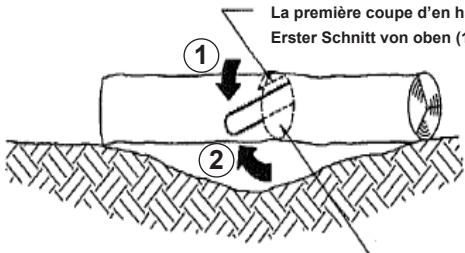
2nd cut underbuck (2/3 diameter) to meet 1st cut (to avoid pinching)
