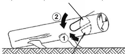
1nd cut underbuck (1/3 diameter) to avoid splintering
